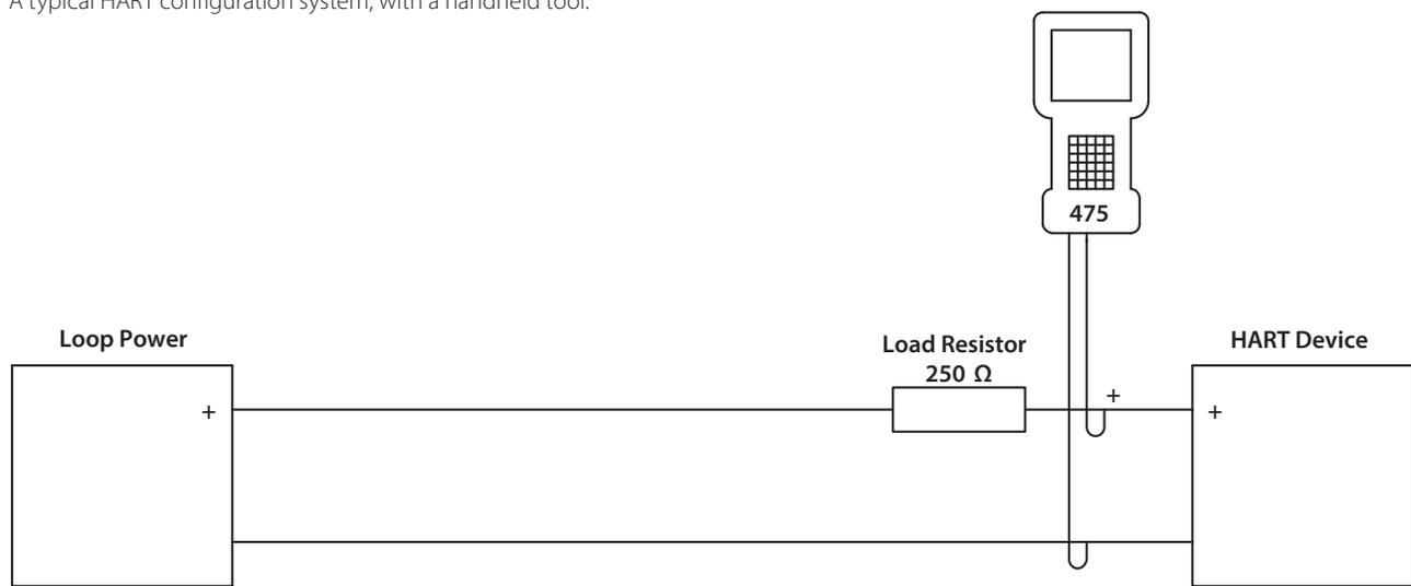
Fig. 2: Typical HART set up with Handheld tool
