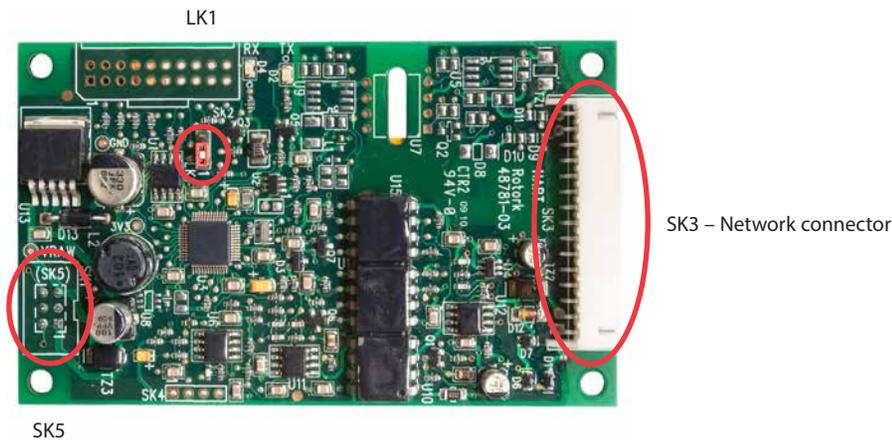
Fig 3 : The HART Field Unit, showing the network connector
