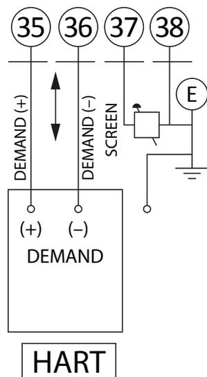
Network connections are made to the terminals of the actuator as defined in the wiring diagram. Shown here is a typical arrangement used in standard wiring diagrams, in this case HART connections here are made to terminals 35 (+) and 36 (-) of the terminal bung. The wiring diagram should be checked to confirm the correct terminal numbers and to confirm which terminal has positive and which terminal has negative polarity.
